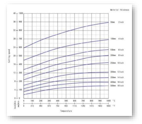
The Above diagrams indicate the cutting speed depending on material thickness and material temperature with a carbon equivalent of max. 0.3%. Homogeneous material microstructure, proper pressure adjustment and purity of oxygen of min. 99.5 % is assumed.
