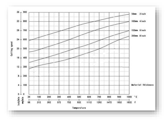
The Above diagrams indicate the cutting speed depending on material thickness and material temperature with a carbon equivalent of max. 0.3%. Homogeneous material microstructure, proper pressure adjustment and purity of oxygen of min. 99.5 % is assumed.
