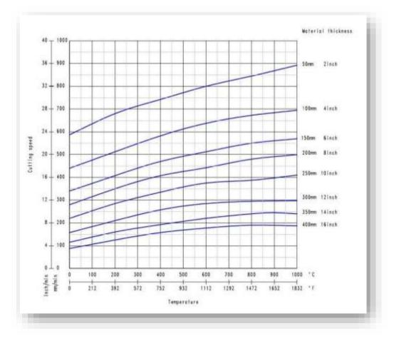
The Above diagrams indicates the cutting speed depending on material thickness and material temperature with a carbon equivalent of max. 0.3%. Homogeneous material microstructure, proper pressure adjustment and purity of oxygen of min. 99.5 % is assumed.
